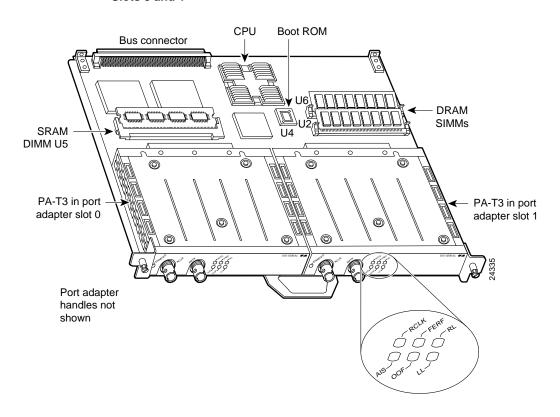
Figure 3-1 VIP2-15 or VIP2-40 with One-Port PA-T3 Serial Port Adapters in Port Adapter Slots 0 and 1
